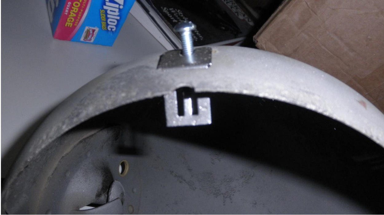
Another view of headlamp retaining bracket installed with screw –
