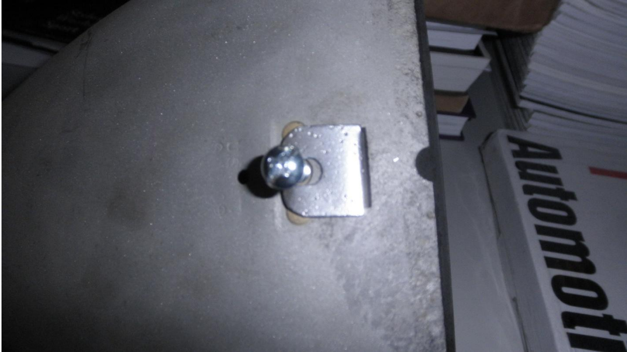
Picture of headlamp retaining bracket and screw installed –
