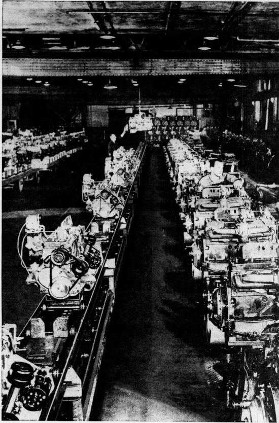
Following assembly of the engines they are "run in," as is pictured, in one of the final testing bays. Here the pulse of the famous Hudson quality-built engines are checked. Their extreme smoothness permits the engines to be tested without being bolted to the stand.
