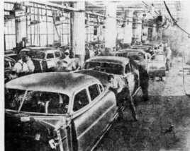
Long trip through oven held at a temperature of 210 degrees. On emerging from the oven, the bodies are inspected for imperfections in the priming coat. A coat of wax is then applied and the conveyor takes the bodies through the industry's finest, most modern spray booths where they receive three double coats of lacquer.
