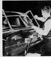
In the case of windshields, the glass is pushed into position from inside the car. Suction cups attached to bracing fixtures on roof above the windshield and on the crest hold it until moldings and weather stripping are installed.
