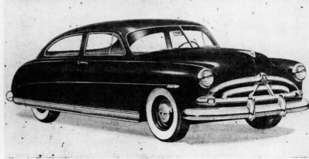
The Pacemaker Custom two-door brougham has a wheelbase of 124 inches. It is powered by the high compression Pacemaker 112 horsepower engine and, like all Hudsons, has exclusive "step-down" design.
