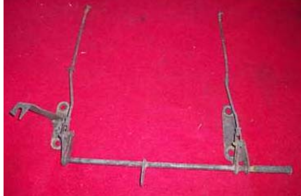
Short Wheelbase Hudson Twin H linkage note the center connection for throttle pedal linkage
