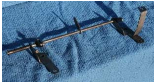
Short Wheelbase Hudson Twin H linkage
