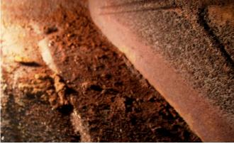
What you see here is what's left of the original screen unit with part of it which has come loose at the right. After years of storing old gas these will no longer be the screen that keeps crud out, but the remnant which keeps crud in which will plug up your intake tube. This tube was so packed with stuff all 3 inches from the end of it had to be drilled out.
